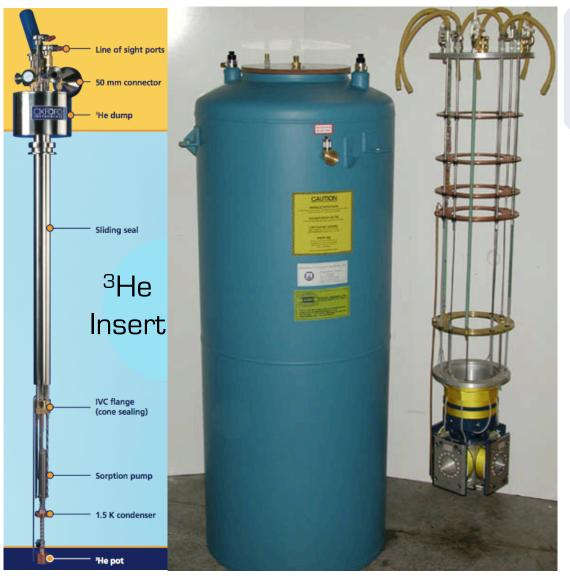
Measurements taken between 0.4 K to 6 K in a <sup>3</sup>He refrigerator with a 3D superconducting vector magnet.
