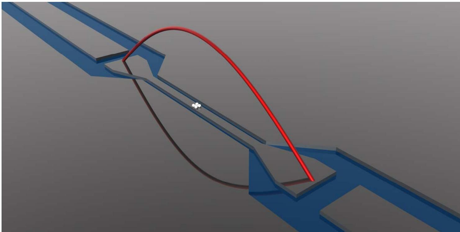
Molecules or diluted spins, placed in the anti-node of an on-chip cavity
