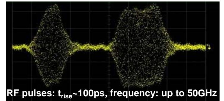
RF pulses:  $t_{rise} \sim 100\text{ps}$ , frequency: up to 50GHz
