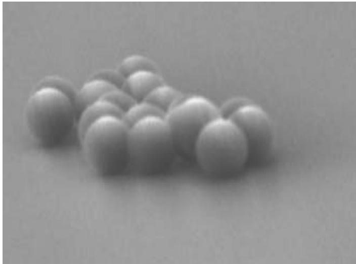
1  $\mu\text{m}$  polystyrene/iron-oxide beads
