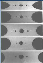
Rayleigh-Plateau instability: Satellite formation in fluids... for lower viscosity higher number of satellites
