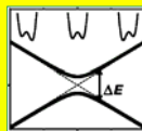
ABOVE: The the energy levels of A SQUID vary as we change the external field. These levels are superpositions of flux states.
