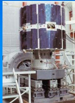
LEFT: The Cos-B satellite under construction. It carries a gamma-ray telescope
